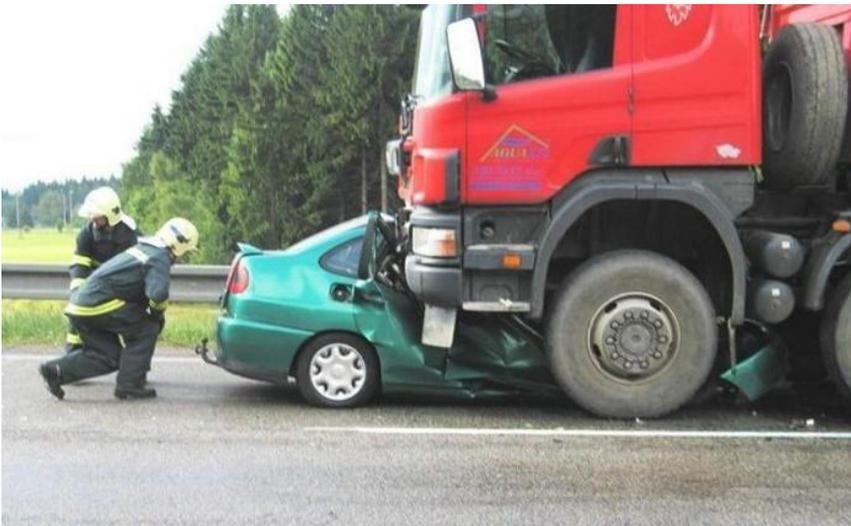
*Example of collision with truck without under-run protection*
